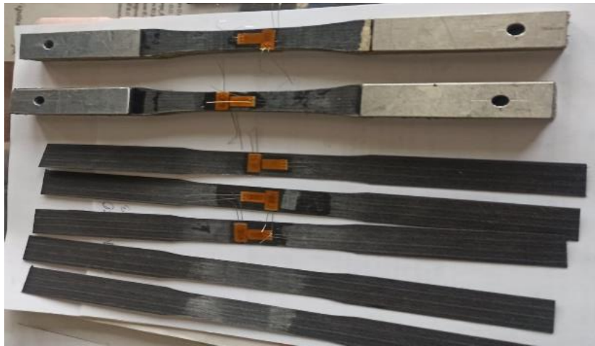
Figure 3 – General appearance of samples before testing.
